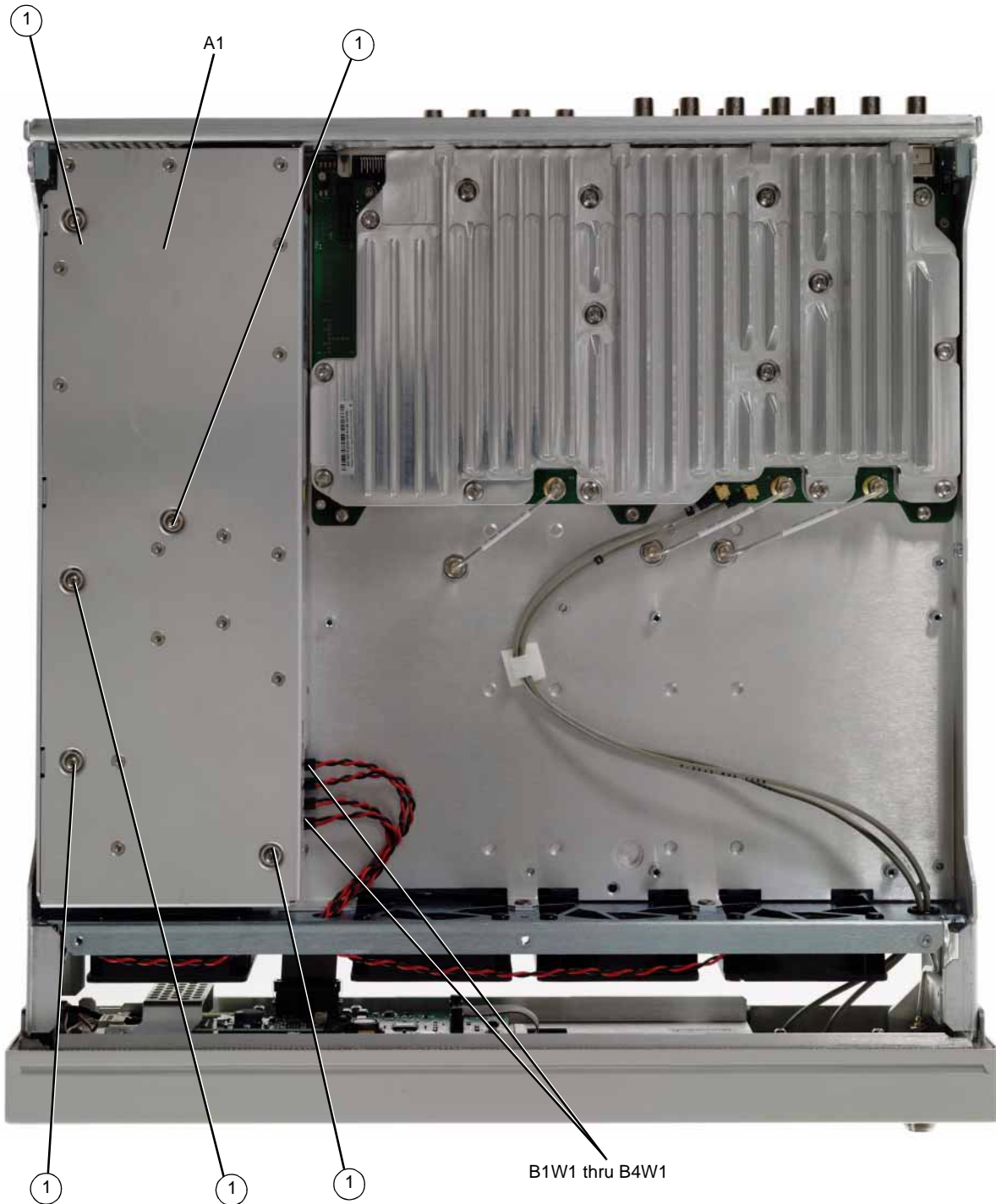
Figure 3-14 A1 Power Supply
